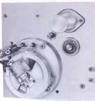
Figure 3. Interior view of the 1362 Oscillator showing new GE Y-1266 planar triode.
